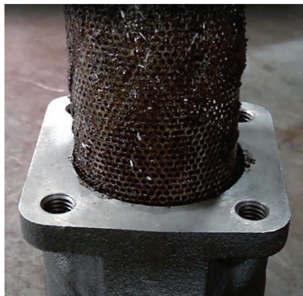
Clogged strainers signal suspended solids, which are a legitimate threat to most process pumps.
